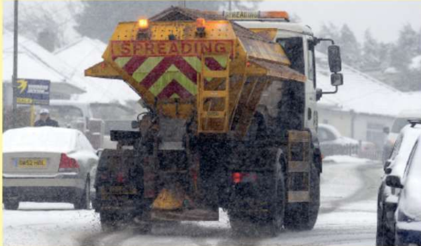
▲ Figure 3.20 Salt gritter at work to prevent ice formation on a road
