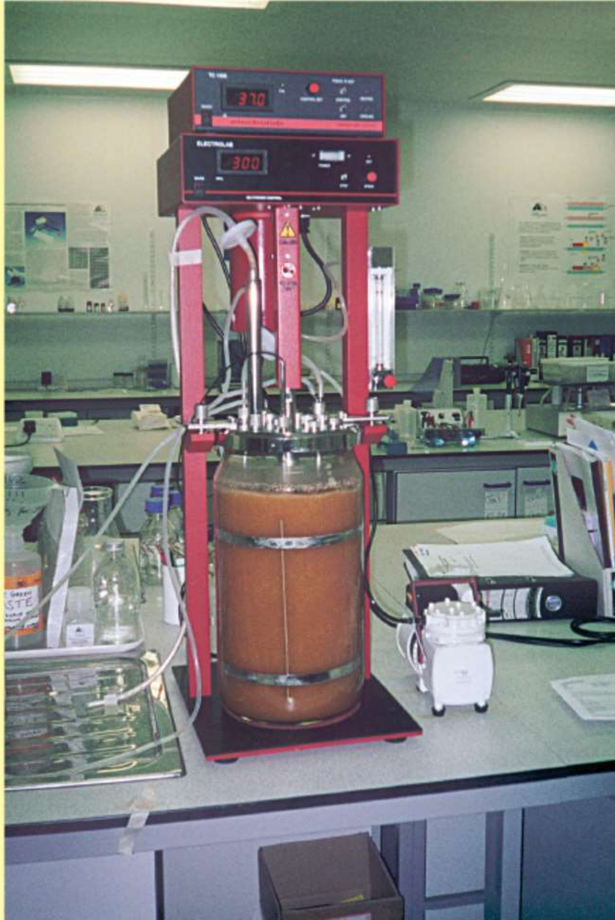
▲ Figure 21.5 A laboratory fermenter for antibiotic production, which will eventually be scaled up to 10 000-litre fermentation vessels
